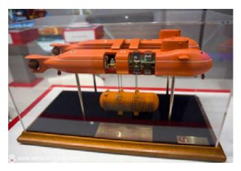
from the Russian Arctic shelf. The advantage of using nuclearpowered submarines are both that they could sail under the ice, thus operate in all weather and ice conditions, as well as function as a platform for placing sub-sea installations on the sea-floor (photo left) and transport minerals to shore port facilities. The set of submarines are powered by a newly developed 24 MW marine reactor. Russian design institutes working on the
