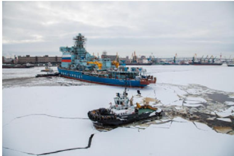
for operation along the Northern Sea Route, presumably for the eastern part from the Taymyr Peninsula towards the Bering Strait where ice conditions normally are more severe (thicker ice) than in the Kara Sea. Maximum icebreaking capability is 3 m. Speed in non-icy waters is up to 22 knots. All vessels of the class have an operational horizon beyond 2039.
