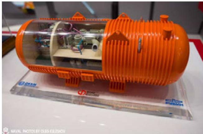
reactor will have an autonomous operation period of at least 8,000 hours providing power to both drilling for petroleum and future mining exploration on the Arctic shelf. The reactor unit is named SHELF is up to 14 meters long and 8 meters in diameter. Reactor core is said to work up to 30 years before the uranium fuel elements have to be reloaded. Depending on design, electric power capacity would range from 8 to 25 MW.
