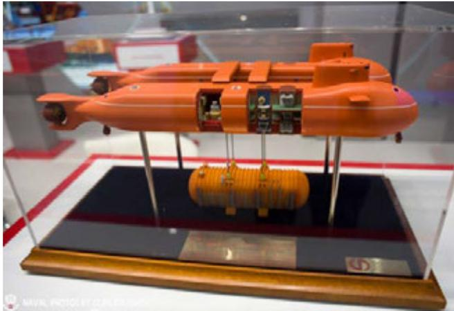
from the Russian Arctic shelf. The advantage of using nuclear-powered submarines are both that they could sail under the ice, thus operate in all weather and ice conditions, as well as function as a platform for placing sub-sea installations on the sea-floor (photo left) and transport minerals to shore port facilities. The set of submarines are powered by a newly developed 24 MW marine reactor. Russian design institutes working on the
